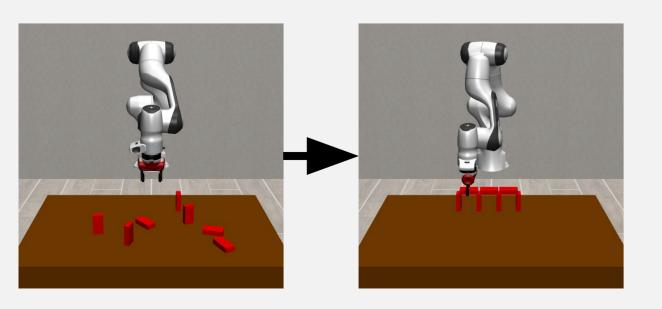
Building: The robot's task is to construct a bridge by assembling the building blocks.
